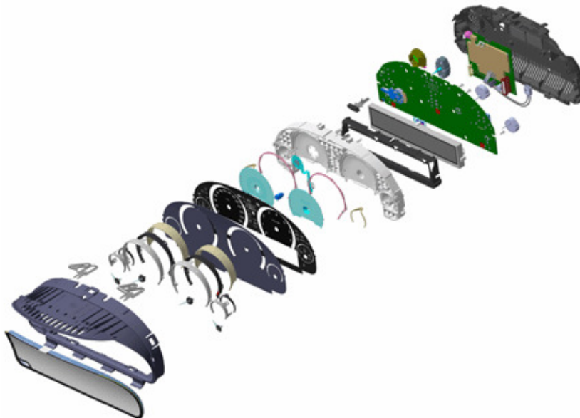
Figure 3: Instrument cluster with 2-printed circuit board concept
