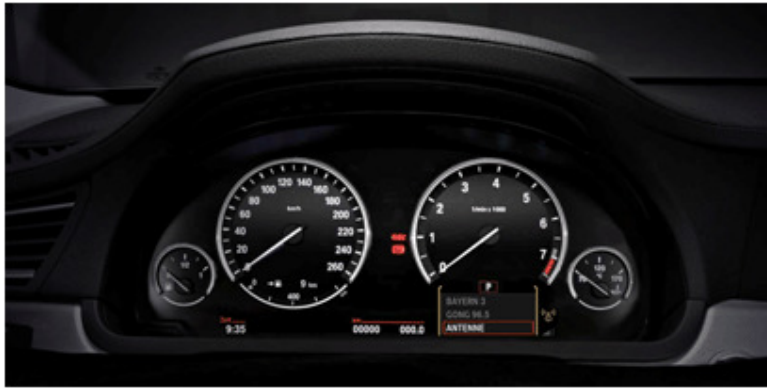
Figure 2: Integrated 9.2" TFT display with super-high contrast red/white LED backlighting
